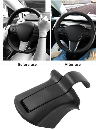
Figure 1: Weight for the steering wheel to trick Tesla’s torque sensor (source: Ali Express)
