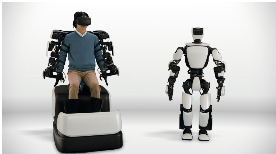
Figure 11.19 The T-HR3 robot (2017–present) can be remotely controlled using a dedicated user interface. (Source: Toyota)
