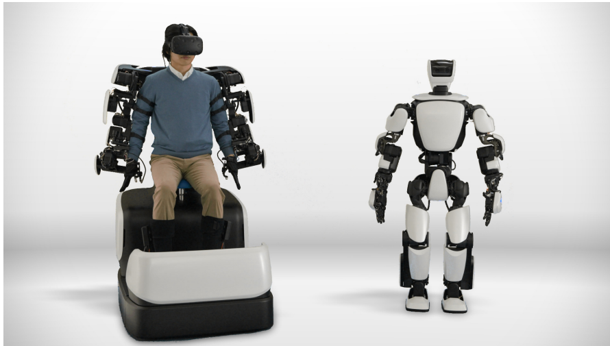
Figure 10.14 The T-HR3 robot (2017–present) can be remotely controlled using a dedicated user interface. (Source: Toyota)
