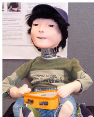
Figure 9.2 Kaspar (2009– present) is a “minimally expressive” robot, built using brackets, servo motors, and a surgical silicon mask. Kaspar is used in autism therapy. (Source: Kerstin Dautenhahn, Ben Robins, Adaptive Systems Research Group, University of Hertfordshire, UK)
