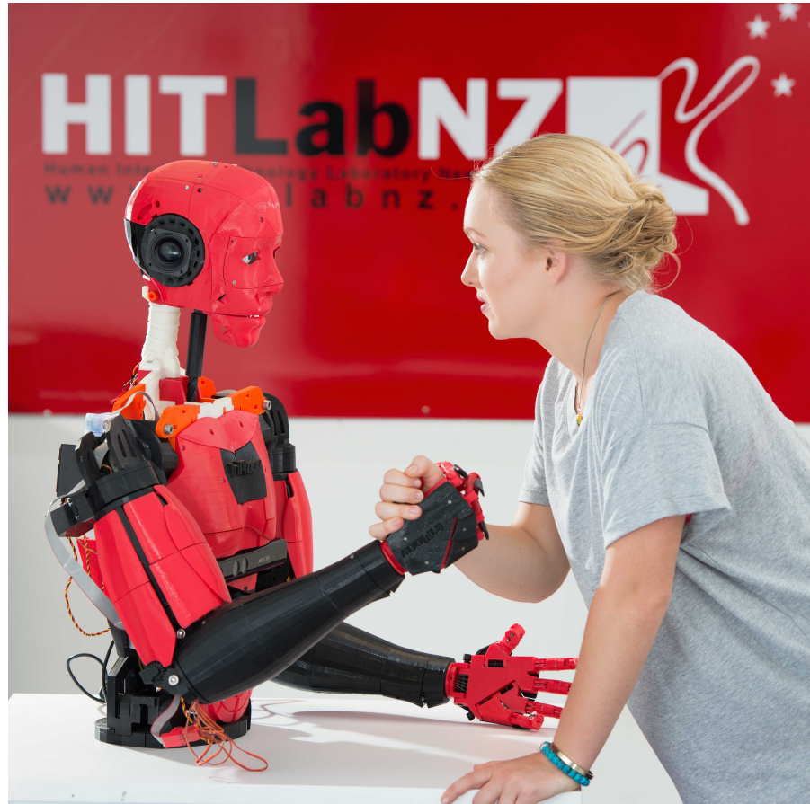
Figure 2.8 InMoov (2012–present) can be built using rapid-prototyping technology and readily available components. The InMoov robot is an open-source social robot.
