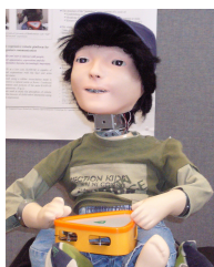
Figure 2.9 Kaspar (2009–present) is a “minimally expressive” robot, built using brackets, servo motors, and a surgical silicon mask. Kaspar is used in autism therapy.
